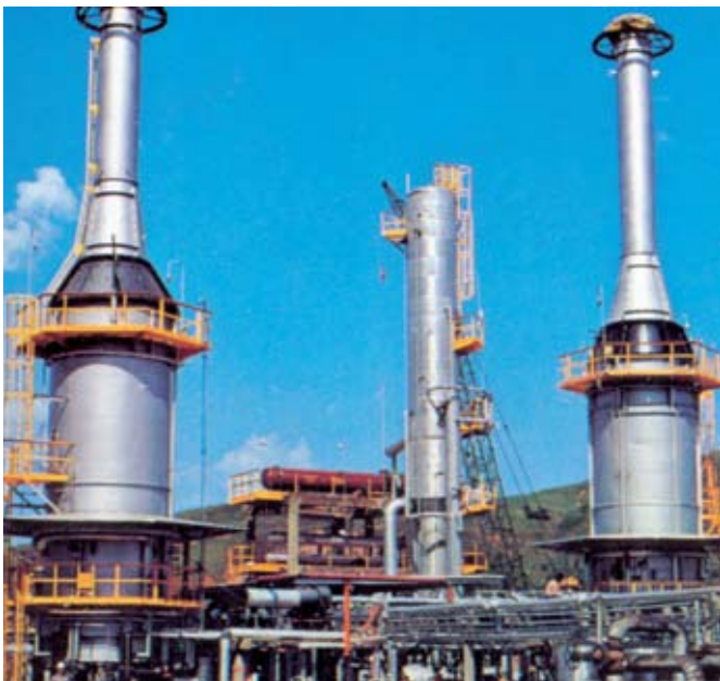
▼ Cylindrical fired heaters.
