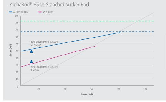
AlphaRod® HS sucker rods operated with +47% max operative stress in comparison with standard D alloy sucker rods, to achieve +128% gross production.
