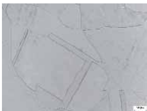
Fig.1 Microstructure of a tube ODxWT 50.8x10.3mm Left: Optical Microscope; Right: Transmission Electronic Microscope
